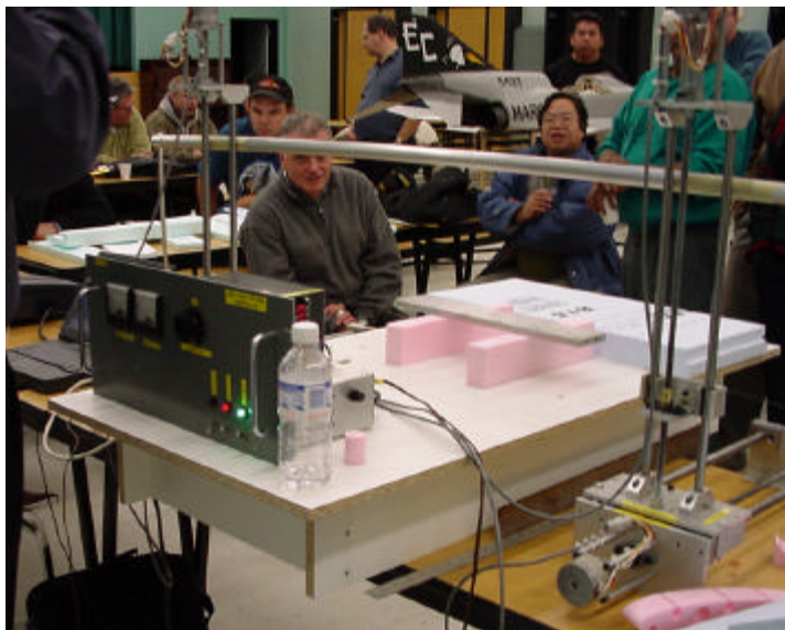
Richard's foam cutting machine; note the computer on the far left, and Don's Phantom in the background.
