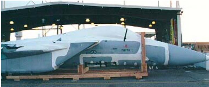
An F-15 being crated up for a customer. Note the white spraylat coating. Wealthier RCFCT members might be interested to know that everything here is for sale.
