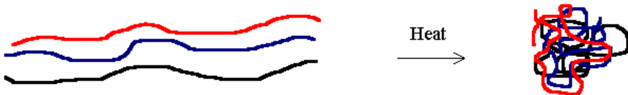
The covering film has stretched out polymer molecules (left), which, when heated, revert to the natural tangled form (right), causing the film to shrink.
