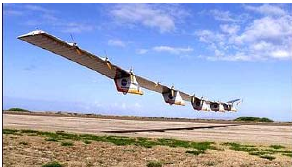
The Helios, a NASA experimental aircraft, uses solar panels on the upper wing surface and can reach an altitude of 100,000 feet. Its wingspan exceeds that of a 747. Like most of our model planes, it is remotely piloted, and covered with plastic film. A discussion of plastic film covering appears on page 5.
