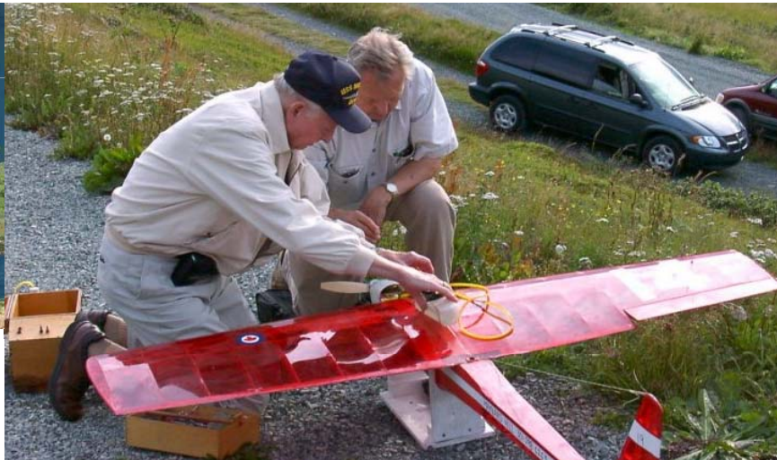
Above: X marks the spot where flight # 3 ended, 479 miles out into the ocean. Right: Roy Day and Maynard Hill (right) prepare for flight #1. Constructed of balsa and mylar film, the plane carries fuel in the wings, and utilizes only 1 aileron.
