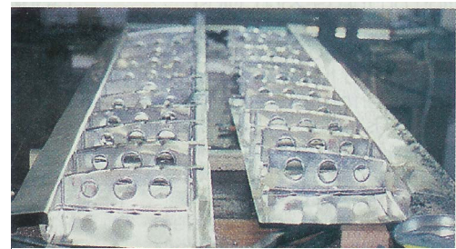
Above: the basic wing structure contains flared lightening holes in the ribs. Left: this all metal scale model of a STOL aircraft looks real enough – but notice that it's sitting on a car roof.
