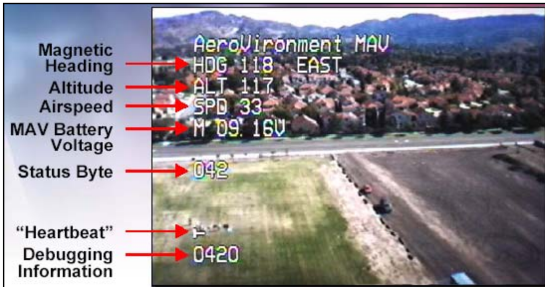
This is a screen shot from the in-flight video feed of a flight of the “Black Widow”, a tiny RC airplane about the size of your hand known as a “MAV” (Micro Aerial Vehicle). Details about this and other unusual RC aircraft appear on page 5.
