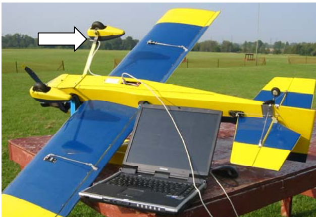
Here's the setup I used – a simple access hatch at the bottom of the plane lets me record the data onto the computer. The arrow shows the location of the pitot tube near the left wheel pant.
