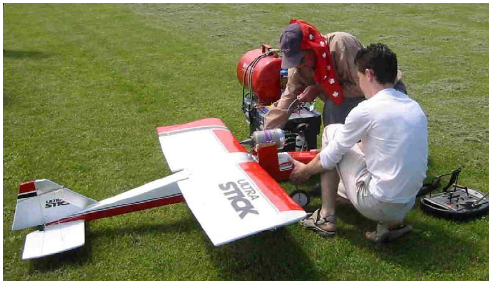
Assisted by Yuri Agayan, Jack Humphries (with hat) prepares to fire up his gas turbine powered Hanger 9 Ultra Stick, at the RCFCF Fun Fly, June 21. Note the aluminum covered fin to protect against the hot exhaust. The sight and sound of this plane in the air was simply awesome. More club associated events on page 3.
