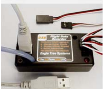
The beige cable hooks up to your computer, and the blue tubing that looks like fuel line connects to the pitot tube
