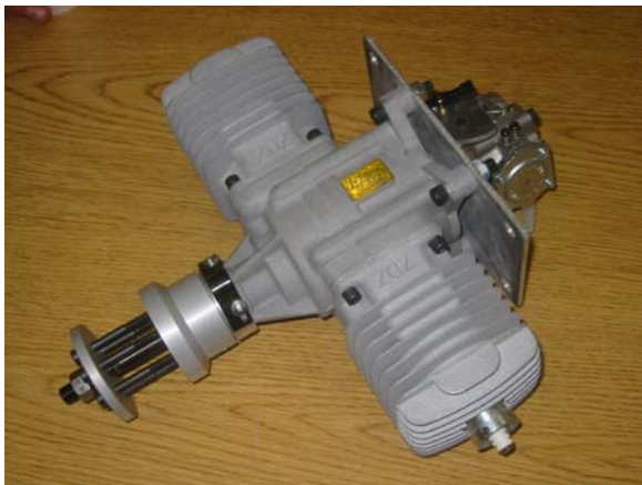
Ron Chapman brought in this fantastic ZDZ160 2 cycle gas engine. This unit can develop over 100 lbs of static thrust!
