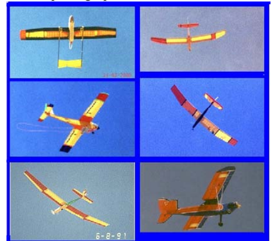
Shown above is the effect of the sun glowing through transparent covering material on open structures. The patches on the Kadet (bottom right) look effective, if a little small.
