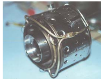
The combustion chamber is typically constructed of stainless steel
