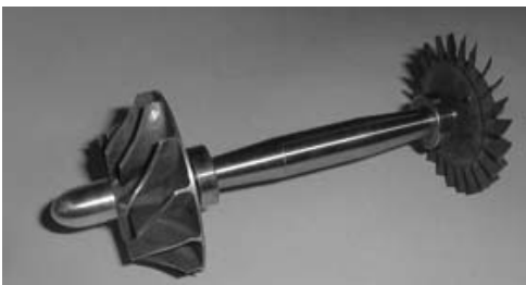
A compressor - turbine assembly.
