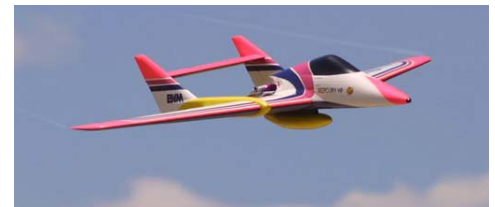
A BVM Bobcat, constructed primarily of composite materials
