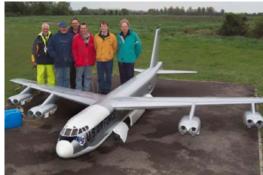
This B-52 is powered by eight Wren MV54s
