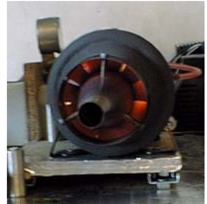
This rear view of a running gas turbine on a test stand suggests that yes, the exhaust is rather warm....
